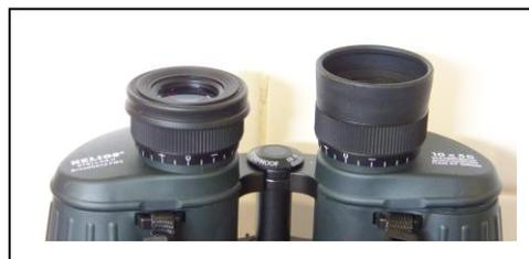
The lens coatings seem to be evenly applied and reduce the amount of reflected light. The manufacturer specifies that the optical transmission is 85%; this seems to be a realistic value. The insides of the objective tubes are ribbed along their entire length, suggesting that control of stray light should be good.
