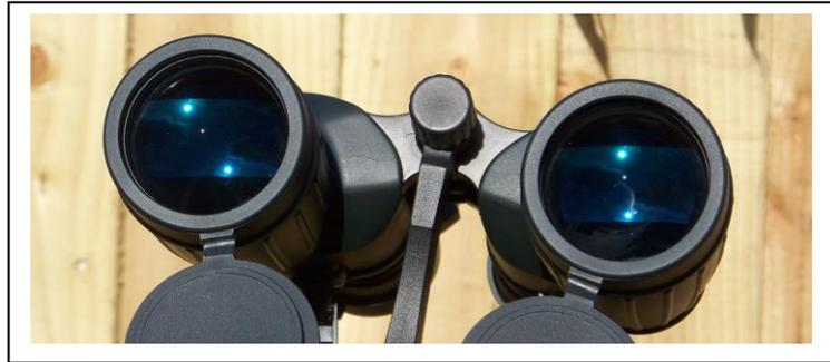
There are is an obvious cut-off segment in each of the light paths, indicating that one of the prisms is slightly undersized, but not so much as to noticeably dim the image. The prisms do not appear to have grooved hypotenuses.
