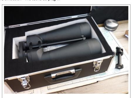
The binocular is also provided with a very substantial metal post-type tripod adaptor that clamps to the mounting bar, where it is secured with two knurled thumb-screws. These are just large enough to be operated with thin-to-medium gloves, but not with thick ones. The bottom of the post is threaded with %-inch Whitworth mounting hole. A %-inch adaptor is thoughtfully included, so that the mounting post will mate with a variety of mounting options.
