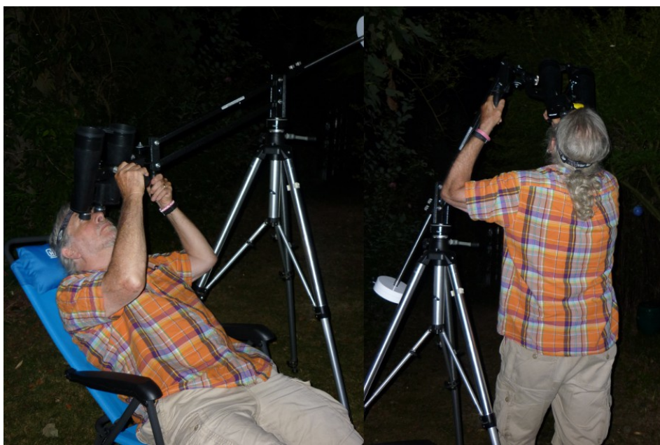
The parallelogram can be used reclined or standing without adjusting the tripod height
