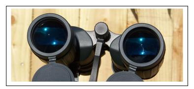
There are is an obvious cut-off segment in each of the light paths, indicating that one of the prisms is slightly undersized, but not so much as to noticeably dim the image. The prisms do not appear to have grooved hypotenuses.
