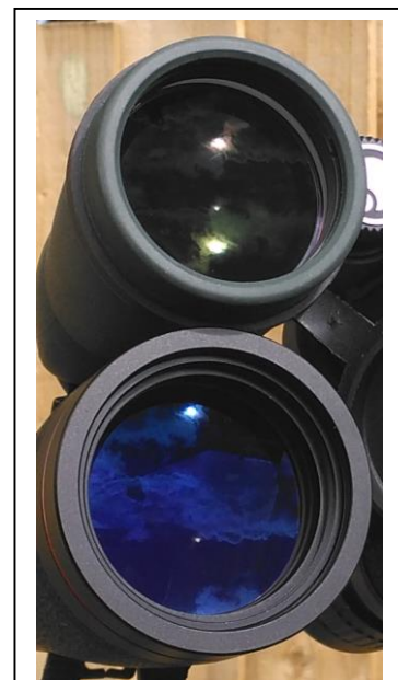
The coatings (above) reflect a small amount of light, but more than a premium binocular (below)
