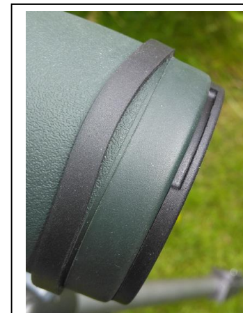
Notches in the rim of the objective caps assist their removal
