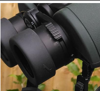
Large lugs aid the right eyepiece adjustment
