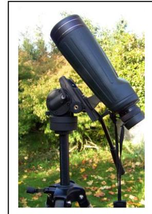
With the centre-column fully extended, the eyepiece height was 182 cm (my eye-height is 165 cm), falling to 161 cm when the binocular was pointed vertically. I found that I could observe comfortably to about  $60^\circ$  and, at a push up to about  $75^\circ$  (measured with a Wixey angle gauge), but this was not comfortable. And was not sustainable for anything but quick views; if you wish to observe higher than this, you will need a chair or recliner.
