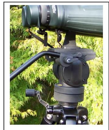
The quick-release plate has a matte finish which causes it to bind slightly when it is being inserted or removed. It has a safety latch to prevent it falling out accidentally if the tightening bolt is left too loose. It is equipped with standard  $\frac{1}{4}$ " and  $\frac{3}{8}$ " Whitworth bolts (slotted for a coin to tighten them) and a video pin.
