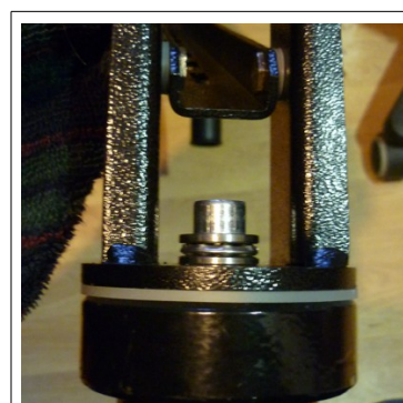
This base-securing bolt can work loose in use; check periodically
