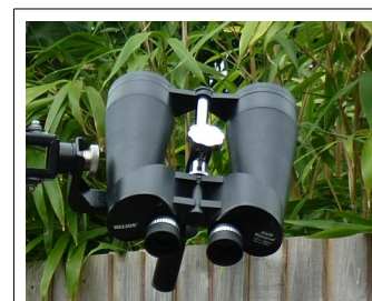
Mounting bar between the optical tubes
