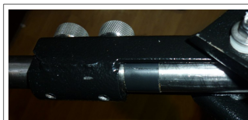
Taped stop on counterweight bar
